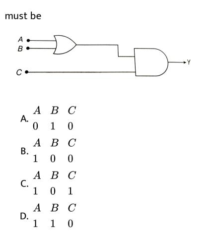
**47.** To get output Y=1 from circuit of figure the input
