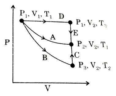
Path A represents a reversible isothermal from  $P_1V_1$  to  $P_2$ ,  $V_2$ , path (B+C) represent a reversible adiabatic expansion (B) from  $P_1, V_1, T_1$  to  $P_3, V_2, T_2$  followed by reversible heating of the gas at
