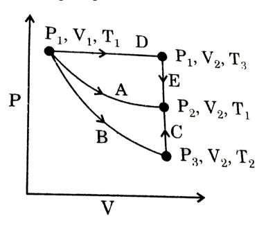
Path A represents a reversible isothermal from  $P_1V_1$  to  $P_2$ ,  $V_2$ , path (B+C) represent a reversible adiabatic expansion (B) from  $P_1, V_1, T_1$  to  $P_3, V_2, T_2$  followed by reversible heating of the gas at constant volume (C) from  $P_3, V_2, T_2$  to  $P_2, V_2, T_1$ . Path (D+E) represents a reversible expansion at constant pressure  $P_1(D)$  from
