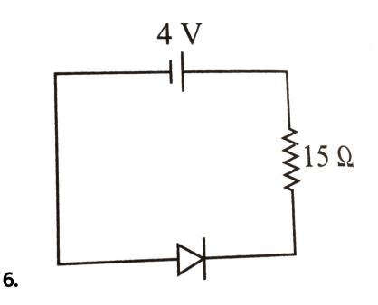
In the circuit shown if current for the diode is  $20\mu A$ , the potential difference across the diode is
