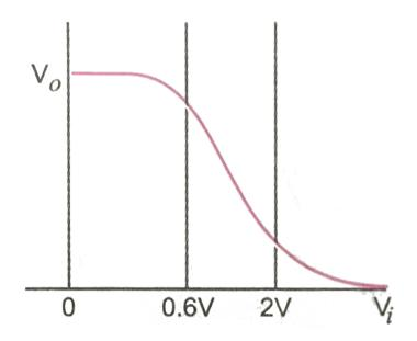
A. At  $V_i=1V$ , it can be used as an amplifier
