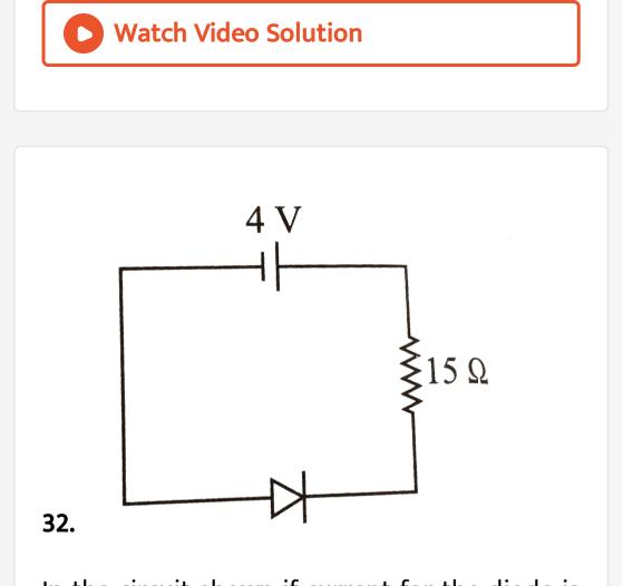
In the circuit shown if current for the diode is  $20\mu A$ , the potential difference across the diode is
