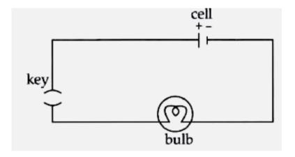
If the bulb is glowing then what will be the direction of the conventional current in the circuit?
