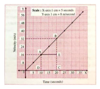
The changes in the velocity of a car in specific time intervals are given in the following table. Explain For all uniformly accelerated motions, the velocity-time graph is a straight line.
