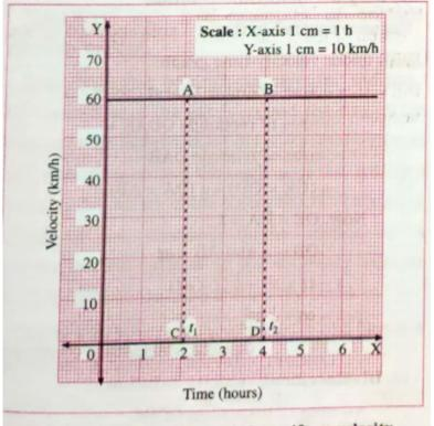
Fig. 1.4 : Velocity-time graph for uniform velocity
