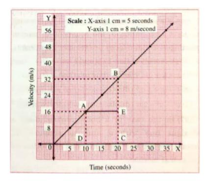
The changes in the velocity of a car in specific time intervals are given in the following table. The velocty-time graph in figure shows that, For nonuniformly accelerated motions, the velocity-time graph may have any shape depending on how the acceleration changes with time.Explain.
