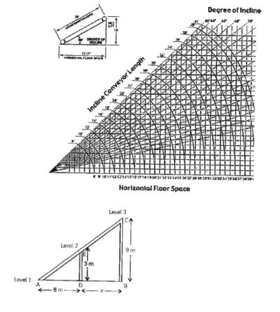
The factory wants to extend the conveyor belt to reach at a new level 3 which is 9 m above level 1 while maintaining the inclination angle.
