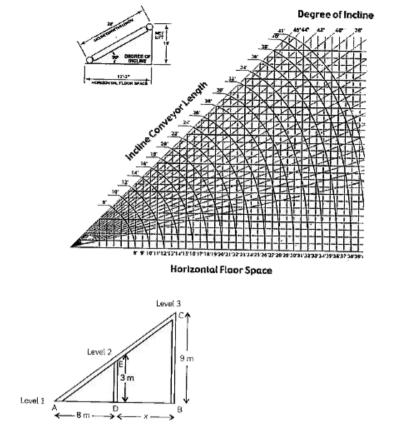
The factory wants to extend the conveyor belt to reach at a new level 3 which is 9 m above level 1 while maintaining the inclination angle. How much distance is extended from D to B? B. 16 m
