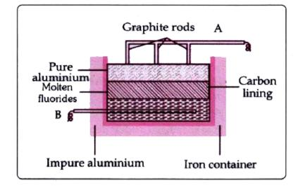
Which of A and B is the cathode and which one is the anode?
