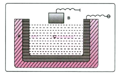
At which electrode (A or B) is the aluminium formed?
