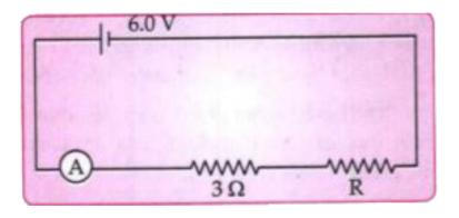
Calculate the value of the unknown resistor R.
