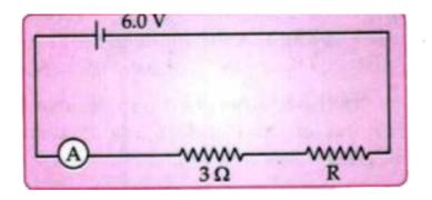
Calculate the power dissipated in the  $3\Omega$  resistor.
