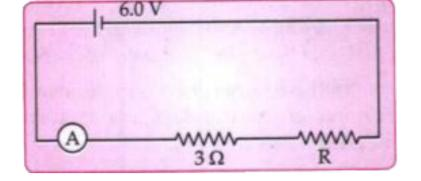
Calculate the value of the unknown resistor R.
