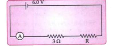
Calculate the charge passing through the  $3\Omega$  resistor in 120 s.
