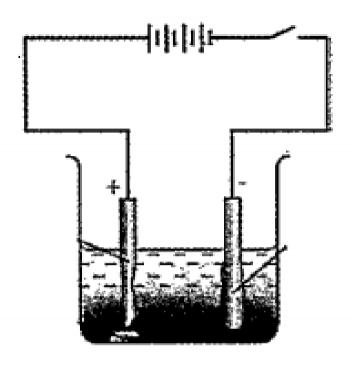
Purification of copper is depicted here: Write the chemical equation during electrolysis.
