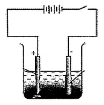
Purification of copper is depicted here: Identify the anode, cathode and electrolyte.
