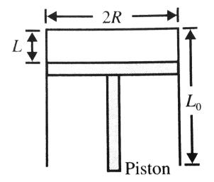
The piston is now pulled out slowly and held at a distance 2L from the top. The pressure in the cylinder between its top and the piston will then be
