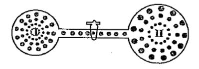
Bulb I has  $2.8gN_2atT_1K$ . The other bulb(II) is completely evacuated. The bulb (I) is heated to  $T_2K$  while bulb (II) is maintained at  $\frac{T_2}{3}K$ . Volume of bulb (I) is half that of bulb (II). If the valve is opened, then what is the weight ratio of  $N_2$  in both bulbs,  $\left(\frac{W_1}{W_2}\right)$ ?
