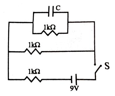
The switch  ${\cal S}$  has been closed for long time so as to charge the capacitor.
