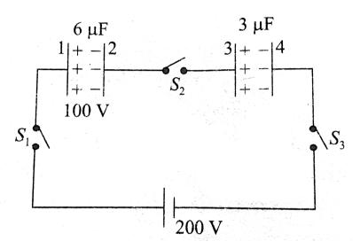
Suppose  $q_1,\,q_2$  and  $q_3$  be the magnitudes of charge flown from switches  $S_1,\,S_2$  and  $S_3$  after they closed. Then
