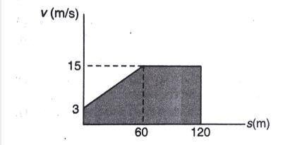
**16.** The jet plane starts from rest at s=0 and is subjected to the acceleration shown. Determine the speed of the plane when it has travelled 60 m.
