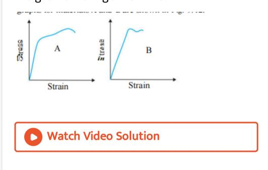
**5.** The stress-strain graphs for materials A and B are shown in Fig. 9.12. Tire graphs are drawn to the same scale ) Which of the two is the stronger material?
