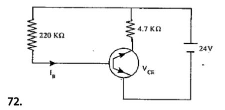
In the above circuit,  $I_C$  =1.5 mA and  $\beta$  = 100.Find  $I_B, V_{CE}$  and  $V_{BE}$
