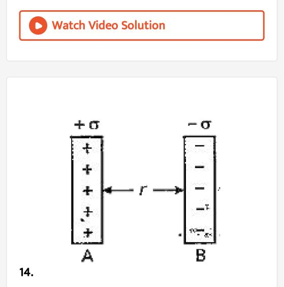
Two large thin metal plates are parallel and close to each other. On their inner surface, plate have surface charge density of opposing magnitude of  $17.0 \times 10^{-22} Cm^{-2}$  as shown. Electric field in outer region of second plate is:
