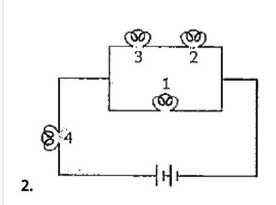
As shown in the figure, four bulb consume same power. The resistance of bulb 1 is  $36\Omega$ . The resistance of bulb 3 is: A.  $9\Omega$
