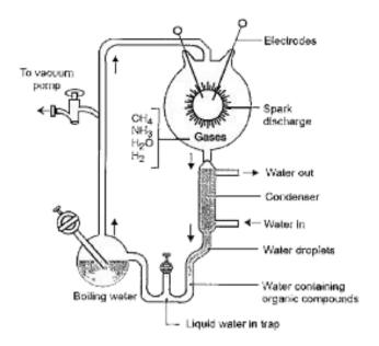
The concept of this experiment is based on
