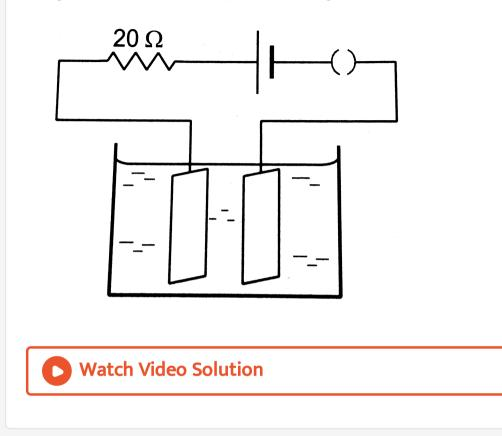
**23.** The potential difference across the terminals of a battery of emf12V and internal resistance  $2\Omega$  drops to 10V when it is connected to a silver voltameter. Find the silver deposited at the cathode in half an hour. Atomic weight of silver is  $107.9gmol^{-1}$ .
