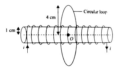
A current 't' in the solenoid results in magnetic field along its axis with magnitude  $B=(\mu)ni$  at points well inside the solenoid on its axis. We can neglect the insignificant field outside the solenoid. This results in a magnetic flux  $(\phi)_B$  through the circular loop. If the current in the winding of solenoid is changed, it will also change the magnetic field  $B=(\mu)_0 ni$  and hence also the magnetic flux through the circular loop.
