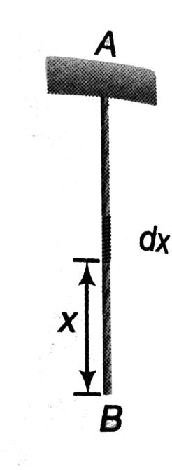
**19.** A rod has a radius of 100 mm and a length of 10 cm. A 100 N force compresses along its length . Calculate the longitudinal stress developed in the rod.
