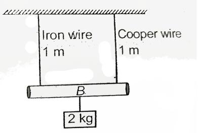
At what distance from iron wire a weight can be hung to produce equal stress in wires?
