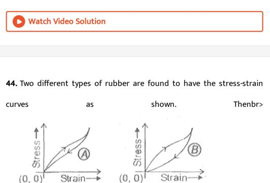
A. A is suitable for shock absorber
