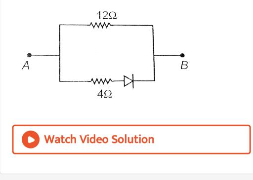
5. The diode used in the circuit shown in the figure has a constant voltage drop of 1V at all current and a maximum power rating of 100mW. What should be the value of the resistor R, connected in series with the diode
