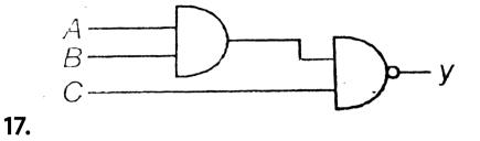
The output y, when all three inputs are first high and then low, will respectively be
