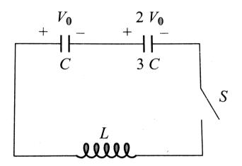
Potential difference across capacitor of capacitance C when the current in the circuit is maximum is
