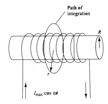
The magnitude of the induced electric field inside tha solenoid, a distance r < R from its long central axis is
