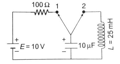
(a) Find the potential across the capacitor after 1s of its connection to position 1. (b) Find the maximum current flowing in the L - C circuit when capacitor is connected across the inductor. Also, find the frequency of LC oscillations.
