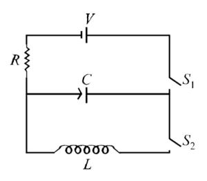
When the capacitor gets charged compleely, (=  $(S_1)$  is opened and  $(S_2)$  is closed, Then,
