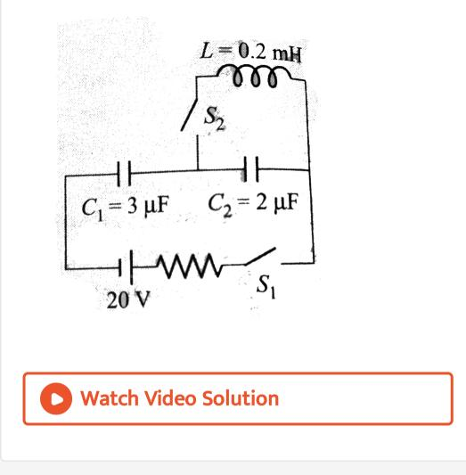
**18.** In the circuit shows in Fig. the battery has negligible internal resistance. Show that the
