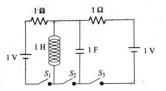
the maximum current in the circuit containing inductor and capacitor (only  $S_2$  is closed)
