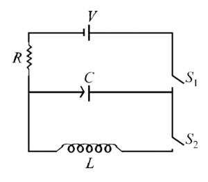
Given taht the total charge stored in the LC circuit is  $(Q_0)$ . for `Tge0, the charge on the capacitor is
