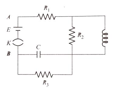
At  $t o \infty$ , the euivalent resistance between A and B is
