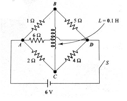
The rate at which the current through the inductor increases initially is
