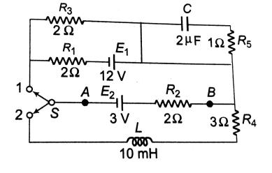
a. The switch S is in position 1. Find the potential differecne  $V_A - V_B$  and the rte of production of joule heat in  $R_1$ b. If now the switch S is put in position 2 at t = 0. Find ItbRrgt i steady current in  $R_4$  and ii hte time when current in  $R_4$  is half the steady value. Also calculate the energy stored
