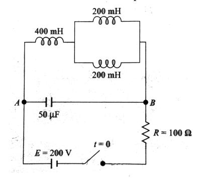
Find the maximum potentail difference across the plates of the capacitor after the switch is opened.
