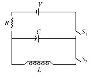
At the start, the capicitor was uncharged. when switch  $(S_1)$  is closed and  $(S_2)$  is kept open, the time constant of this circuit is  $\tau$ . which of the following is correct
