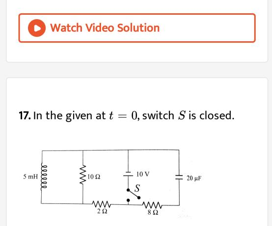
The current through the  $10\Omega$  resistor at any instant  $t(0 < t < \infty)$  will be
