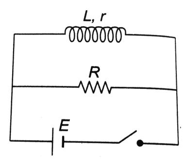
A. Current in the inductor just after removing the battery is  $\frac{E(r+R)}{rR}$ B. Total enery dissipated in the solenoid and the reistor long time after removing
