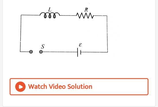
8. In the circuit shows in Fig. the inital current through the inductor at t = 0 is  $I_0$ . After a time t = L/R, the switch is quickly shifted to position 2.
