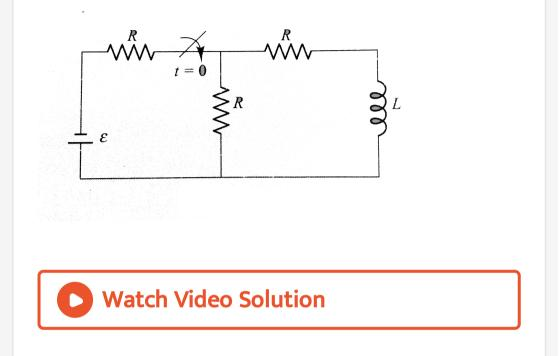
**11.** Figure shows a circuit consisting of an ideal cell, an inductor L, and a resistor R, connected in series. Let switch S be closed at t = 0. Suppose at t = 0, the current in the
