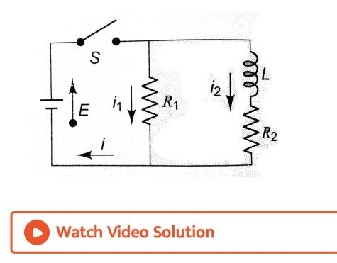
10. In Fig. the switch is closed and steady-state conditions are established. The switch is thrown open at t=0.
