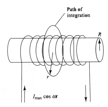
The magnitude of electric field outside the solenoid at a distance r>R from its long central axis is
