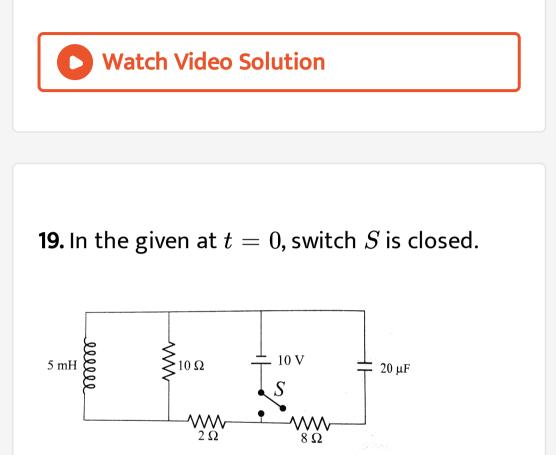
The energy stored in the capacitor and inductor, respectively, at  $t o \infty$  will be
