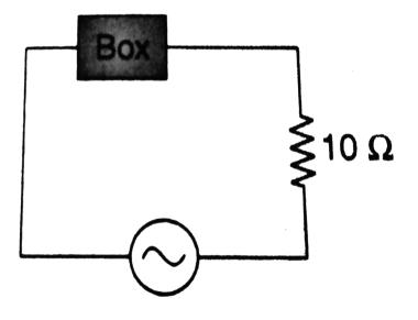
**6.** A circuit element shown in the figureure as a box is having either a capacitor or an inductor. The power factor of the circuit is 0.8, while current lags behind the voltage. Find
