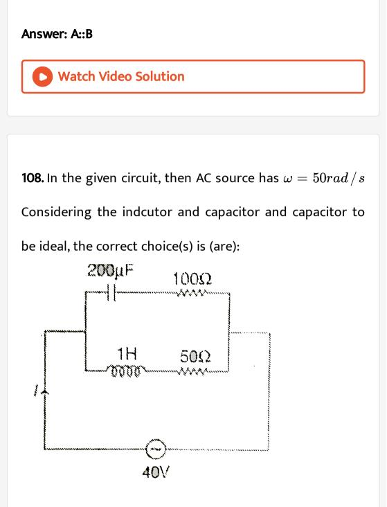
A. The voltage across  $100\Omega$  resistor  $20\sqrt{2}V$
