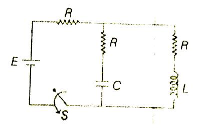
A. after a long time interval potential differences across capacitor and inductor will be equal
