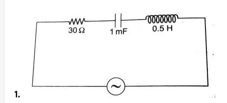
In the diagram shown in figure, V function is given. Find other four functions of time  $I, V_C, V_R$  and  $V_L$ . Also, find power consumed in the circuit, V is given in volts and  $\omega$  in rad/s.
