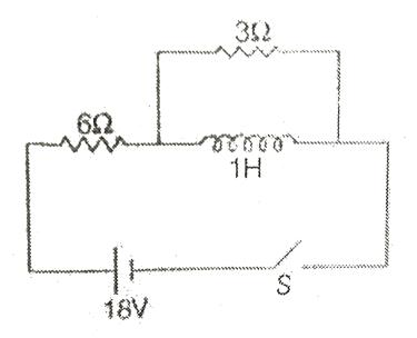
At what time current through  $3\Omega$  resistance and 1H inductor are equal?
