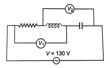
A. Voltage across resistor, inductor and capacitor are 50V, 86.6V and 206.6V respectively B. Voltage across resistor, inductor and capacitor are
