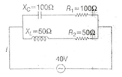
A. The voltage across  $100\Omega$  resistor  $20\sqrt{2}V$
