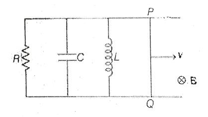
Currents through resistor, capacitor and inductor at any time t are  $l_1$ ,  $I_2$  and  $I_3$  respectively. Current through wire PQ is I.
