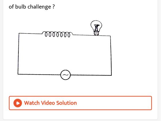
**39.** A light bulb has the rating 200W 220V. Find (i) resistance of the bulb filament (ii) rms value of current flowing through the filament.
