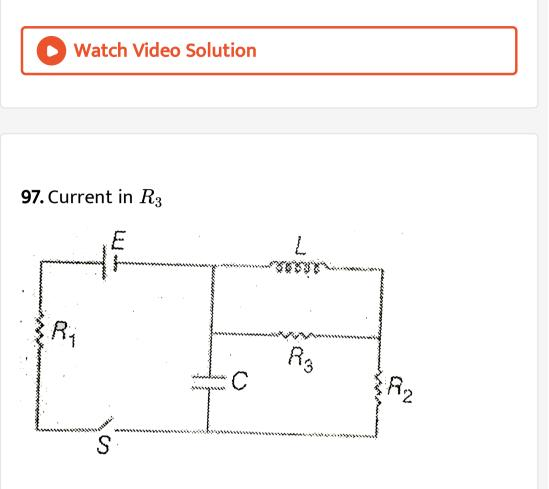
A. just after closing the switch is zero
