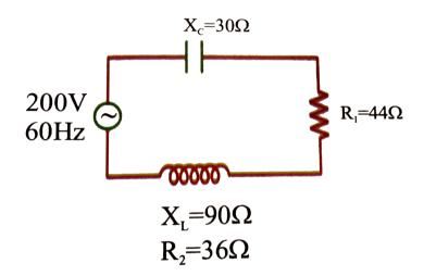
The power dissipated in the inductance coil is
