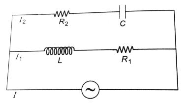
$R_1 = 30\Omega, R_2 = 40\Omega, L = 0.4H$  and  $C = \frac{1}{3}mF$ . Find seven function of time  $I, I_1, I_2, V_{R_1}, V_L, V_{R_2}$  and  $V_C$ . Also total power consumed in the circuit. In the given potential function V is in volts and omega rad/s V=200 sin(100t+30)
