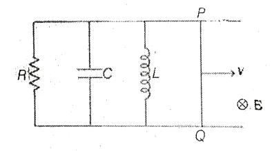
Currents through resistor, capacitor and inductor at any time t are  $l_1$ ,  $I_2$  and  $I_3$  respectively. Current through wire PQ is I.
