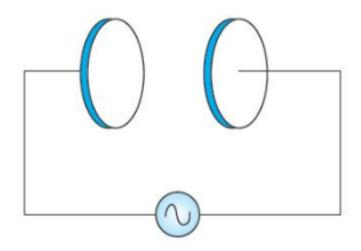
**1.** A parallel- plate capacitor with plate area A and separation between the plates d, is charged by a constant current i. Consider a plane surface of area A/2 parallel to the plates and drawn summetrically between the plates. Find the displacement current through this area.
