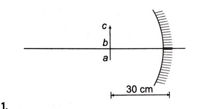
Focal length of the concave mirror shown in figure in 20 cm.
