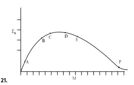
The above is a plate of binding energy per nucleon  $E_0$  against the nuclear mass  $M,\,A,\,B,\,C,\,D,\,E,\,F$  correspond to different nuclei Consider four reactions:
