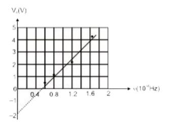
The values of Planks constant and the work function as determined from the graph are (taking the magnitude of electronic charge to be  $e = 1.6 imes 10^{-19} C$ )
