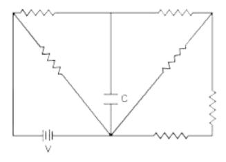
All the resistors are identical. The charge stored in the capacitor, once it is fully charged,
