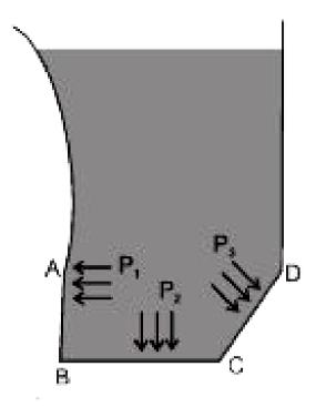
Let  $P_1$ ,  $P_2$  and  $P_3$  be the pressures exerted by the water on the wall AB, base BC and the wall CD respectively. Density of water is  $\rho$  and g is acceleration due to gravity. Then, approximately
