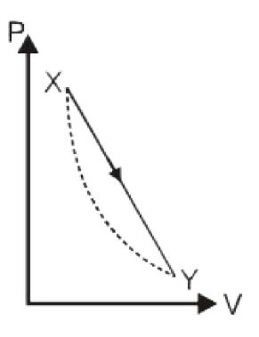
For a process that is described by a straight line joining two points X and Y on the adiabat (solid line in the diagram) heat is : (hint : Consider the variations in temperature from X to Y along the straitght line) A. absorbed throughtout from X to Y B. released throughout from X to Y C. absorbed from X up to an intermediate point Z (not shown in the figure) and then released from 7 to Y D. released from X up to an intermediate point Z (not shown in the figure) and then absorbed from 7 to Y
