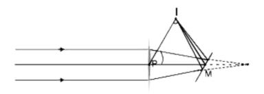
M is a point at which the axis of the lens intersects the mirror. The distance PM is 10 cm.
