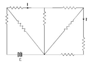
All the resistors are identical. The ratio I/I' is
