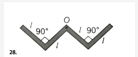
A thin rod of length 4l, mass 4 m is bent at the point as shown in the figure. What is the moment of inertia of the rod about the axis passing through O and perpendicular to the
