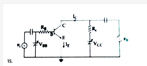
In the figure, given that  $V_{BB}$  supply can vary from 0 to  $5.0V, V_{\mathbb{C}} = 5V, \beta_{dc} = 200, R_B = 100K\omega, R_C = 1K\omega$  and  $V_{BE} = 1.0V$ , The minimum base current and the input voltage at which the transistor will go to saturation, will be, respectively:
