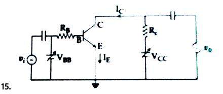
In the figure, given that  $V_{BB}$  supply can vary from 0 to  $5.0V,\,V_{\mathbb C}=5V,\,\beta_{dc}=200,\,R_B=100K\omega,\,R_C=1K\omega$  and  $V_{BE}=1.0V$ , The minimum base current and the input voltage at which the transistor will go to saturation, will be, respectively:
