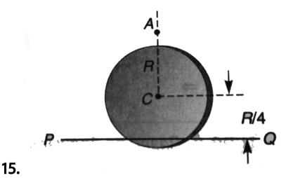
A uniform circular disc has radius R and mass m. A particle, also of mass m, if fixed at a point A on the edge of the disc as shown in the figure. The disc can rotate freely about a horizontal chord PQ that is at a distance R/4 from the centre C of the disc. The line AC is perpendicular to PQ. Initially the disc is held
