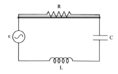
a. Determine the source frequency which drives the circuit in resonance
