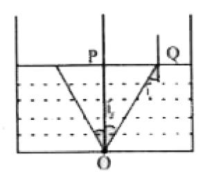
**5.** a.Figure shows a cross-section of a 'light pipe' made of glass fibre of refractive index 1.68
