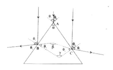
8. A parallel beam of light falls normally on the first face of a prism of small anlge A. At the second face it is partly transmitted partly reflected. The reflected beam striking the first face again, emerges out through the first face at an angle of  $6^{\circ}30'$  with the normal to the first face. The refracted beam is found to hae undergone a deviation of  $1^{\circ}15'$  from the original direction.
