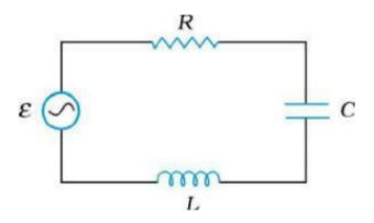
**239.** A resistance of 2 ohm a coil of inductance 0.01 H are connected with a capacitor and put across a 200 V and 50 Hz supply. Calculate the current and voltage across the capacitor at resonance.
