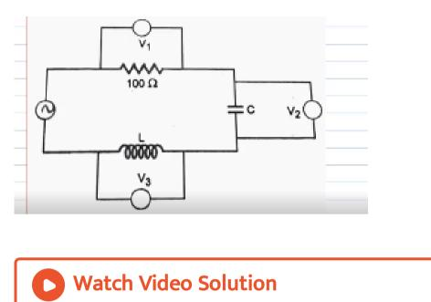
**51.** A series LCR circuit is connected to an a.c. source 220 V - 50 Hz as shown in fig. If the reading of the three voltemeters  $V_1$ ,  $V_2$ ,  $V_3$ are 65 V, 415 V and 204 V respectively R=100 ohm. Calculate value of C for same L required
