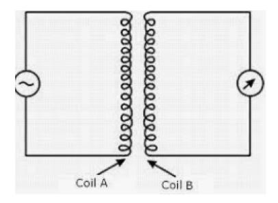
**42.** The circuit arrangement given in the figure shows that when an ac. passes through the coil A, the current starts flowing in the coil B. Mention two factors on which the current produced in the coil B depends.
