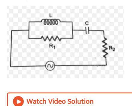
**64.** In the circuit shows find the phase difference between the potential differences across C and  $R_2$
