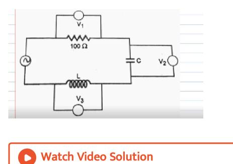
**49.** A series LCR circuit is connected to an a.c. source 220 V - 50 Hz as shown in fig. If the reading of the three voltmeters  $V_1$ ,  $V_2$ ,  $V_3$  are 65 V, 415 V and 204 V respectively. Calculate value of inductor L.
