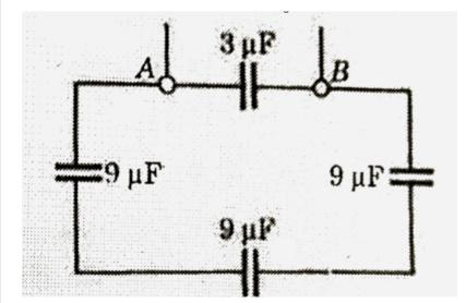
**22.** Find the equivalent capacitance of the combination of capacitons between the points A and B as shown in the figure. Also calcualte the total charge that flows in the circuit, when a 100 V battery is connected between the points A and B.
