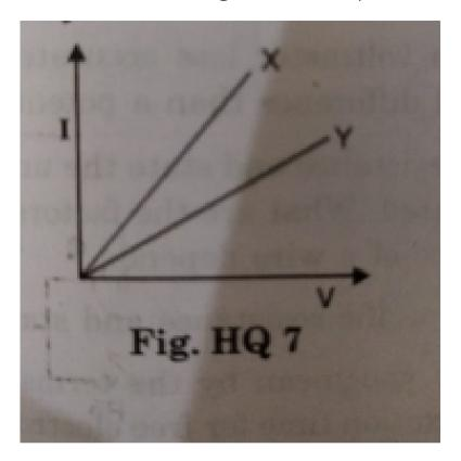
**168.** V-I graph for a mettalic wire at two different temperatures  $T_1$  and  $T_2$  is as shown in figure. Which of the temperatures  $T_1$  and  $T_2$  is higher and why.
