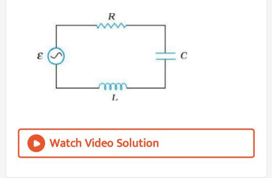
14. Figure shows a series LCR circuit connected to a variable frequency 230 V source. L = 5.0 H,  $C=80\mu F,\,R=40\Omega$ . Obtain the impedance of the circuit and the amplitude of current at
