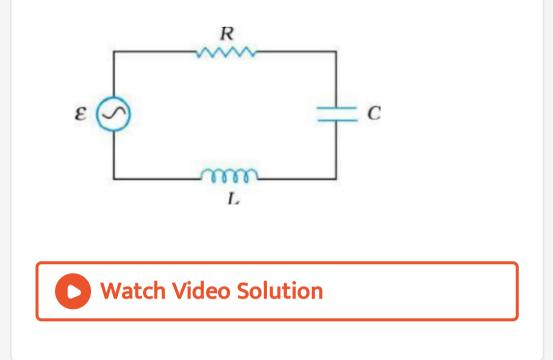
15. Figure shows a series LCR circuit connected to a variable frequency 230 V source. L = 5.0 H,  $C = 80 \mu F$ ,  $R = 40 \Omega$ . Determine the rms potential drops across the three elements of the circuit. Show that the potential drop across the LC combination is zero at the
