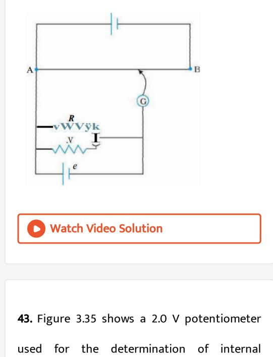
resistance of a 1.5 V cell. The balance point of the cell in open circuit is 76.3 cm. When a resistor of  $9.5\Omega$  is used in the external circuit of the cell, the balance point shifts to 64.8 cm length of the potentiometer wire. Determine the internal resistance of the cell. :
