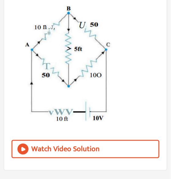
**12.** In a metre bridge [Fig. 3.27], the balance point is found to be at 39.5 cm from the end A,
