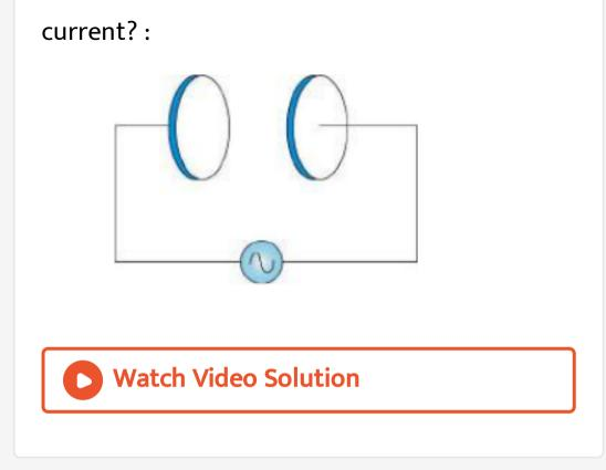
**6.** A parallel plate capacitor (Fig. 8.7) made of circular plates each of radius R = 6.0 cm has a capacitance C = 100 pF. The capacitor is connected to a 230 V ac supply with a (angular) frequency of  $300rads^{-1}$ . Determine the amplitude of B at a point 3.0 cm from the axis between the plates. :
