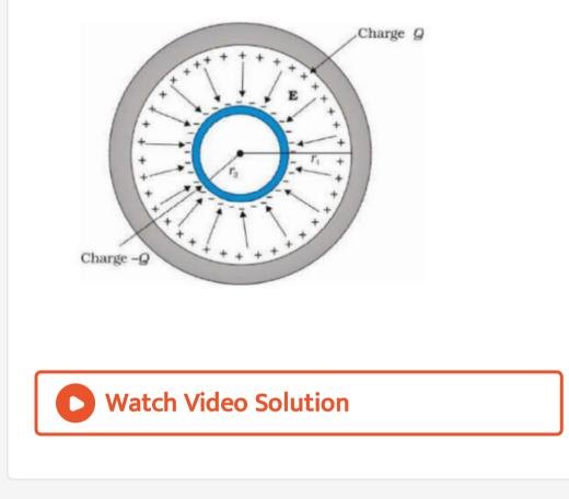
**41.** A spherical capacitor has an inner sphere of radius 12 cm and an outer sphere of radius 13 cm. The outer sphere is earthed and the
