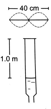
**51.** A 30.0-cm-long wire having a mass of 10.0 g is fixed at the two ends and is vibrated in its fundamental mode. A 50.0-cm-long closed organ pipe, placed with its open end near the wire, is set up into resonance in its fundamental mode by the vibrating wire. Find the tension in the wire. Speed of sound in air  $= 340ms^{-1}$ .
