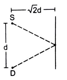
**29.** Two stereo speakers are separated by a distance of 2.40 m. A person stands at a distance of 3.20 m directly in front of one of the speakers as shown in figure. Find the frequencies in the audible range (20-2000 Hz) for which the listener will hear a minimum sound intensity. Speed of sound in air  $= 320ms^{-1}$
