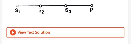
**33.** Two coherent narrow slits emitting sound of wavelength  $\lambda$  in the same phase are placed parallet to each other at a small separation of  $2\lambda$ . The sound is delected by maving a delector on the screen at a distance  $D(>>\lambda)$  from the slit  $S_1$  as shows in figure. Find the distance y such that the intensity at P is equal to
