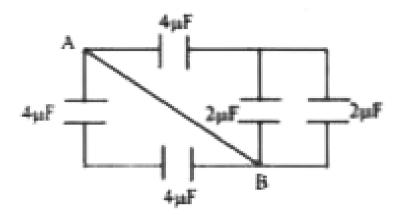
The effective capacitance between A and B is
