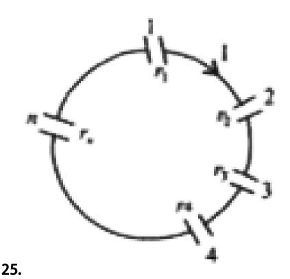
A group of N cells whose e.m.f. varies directly with the internal resistance as per the equation  $E_n=1.5r_n$  are connected as shown in the figure above. The current I in the circuit
