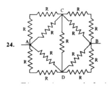
Thirteen resistances each of resistance R ohm are connected in the circuit as shown in the figure above. The effective resistance between A and B is
