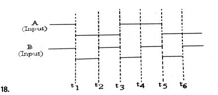
The give inputs A, B are fed to a 2-input NAND gate. Draw the output
