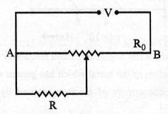
A resistance of R draws current from a potentiometer. The potentiometer wire, AB, has a total resistance of  $R_o$ . A voltage V is supplied to the potentiometer. Derive an expression for the voltage across R when the sliding contact is in the middle of potentiometer wire.
