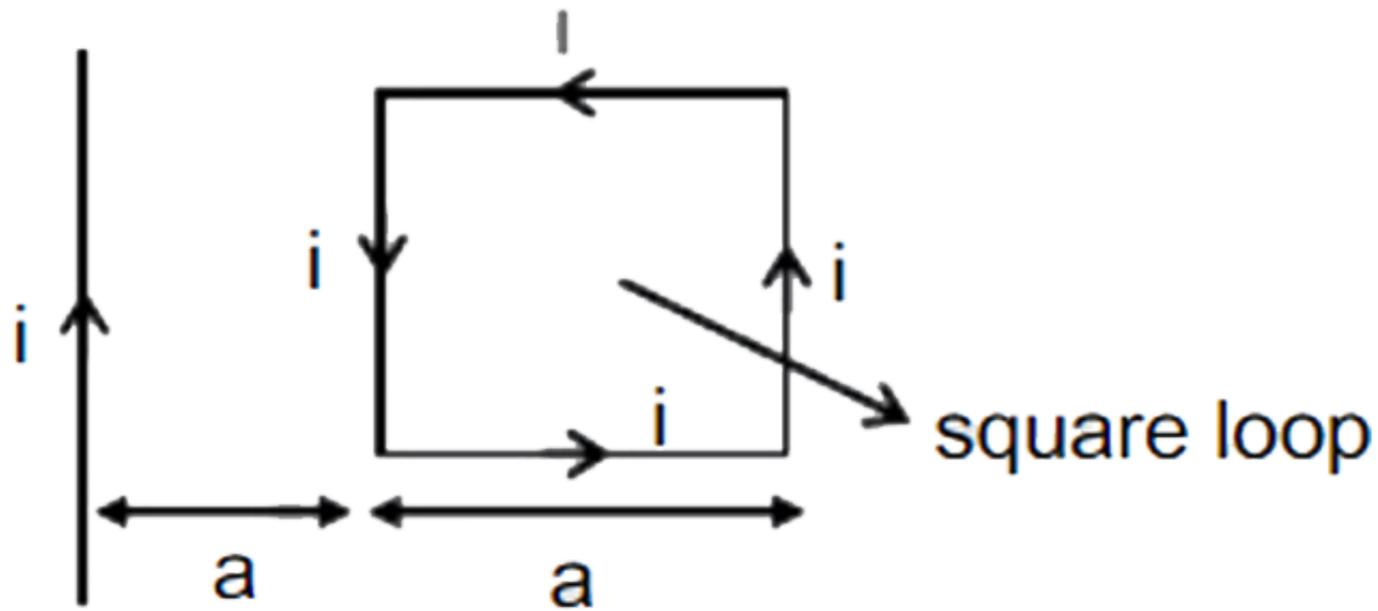
The force between the infinite wire and the square loop is
