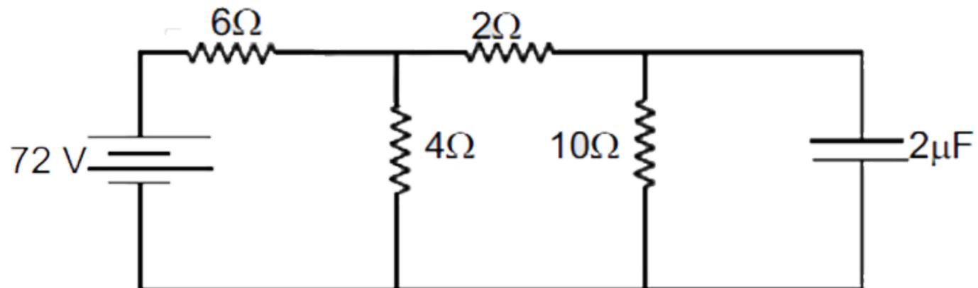
Determine the charge on capacitor in steady state:
