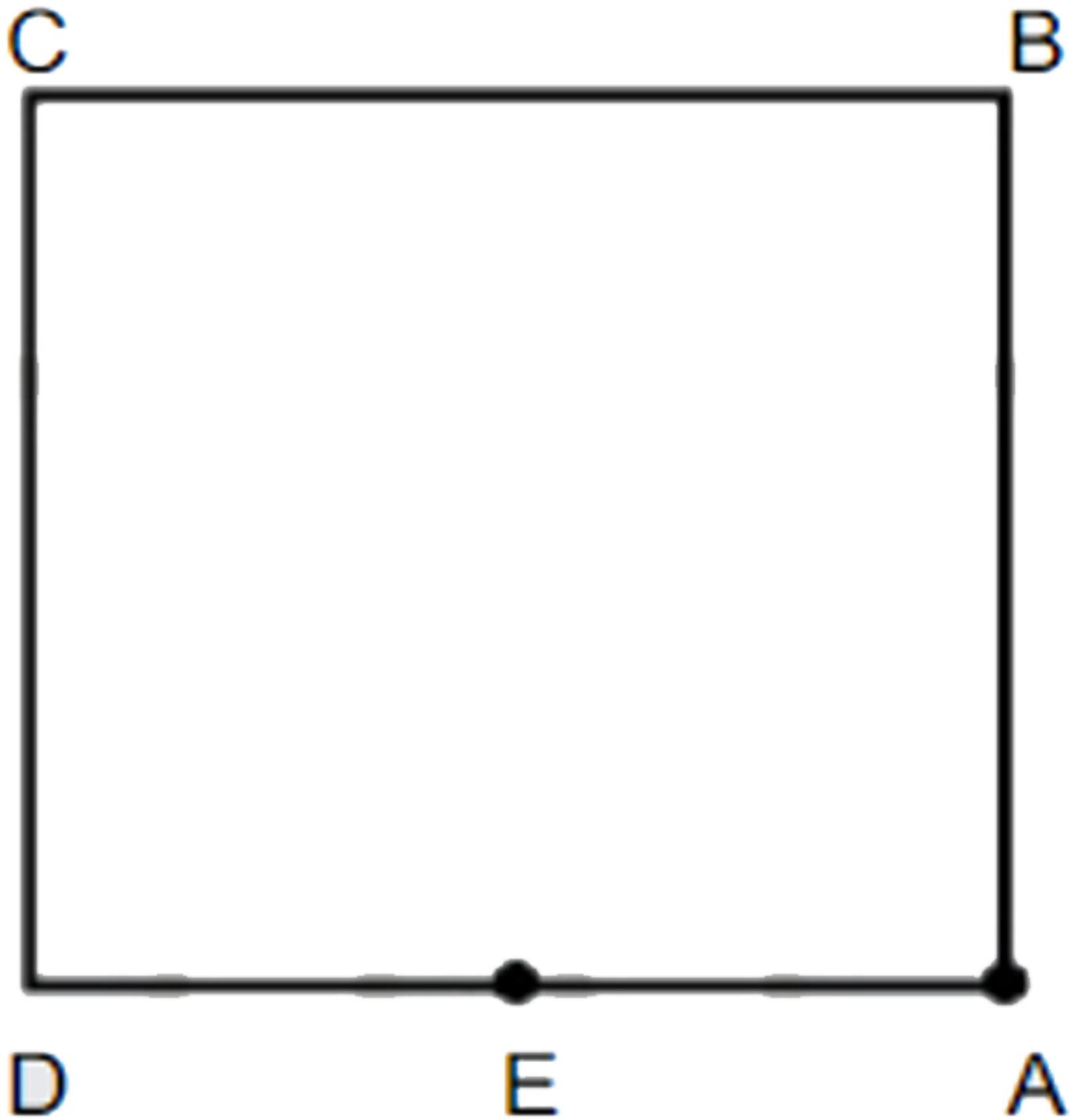
A wire of length  $l$  and resistance  $R$  is bent in form of square form of square as shown in figure. If  $E$  is a mid point of side  $D,A$ , then equivalent resistance between points  $E$  &  $A$  is:
