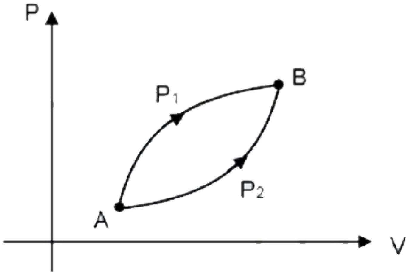
A thermodynamic system undergoes two processes  $P_1$  and  $P_2$  from  $A \rightarrow B$  as shown in  $P - V$  diagram, choose the correct option.
