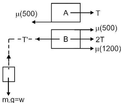
$$3T + 0.3 \times 1200 = m_c g = W \text{ and } T = \mu(500) = 0.3 \times 500$$
