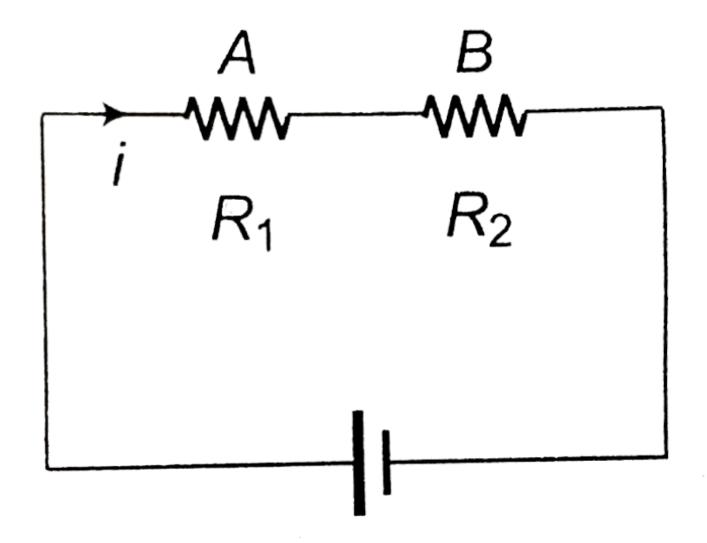
$P_A=i^2R_1, P_B=i^2R_2$  $R_1>R_2\Rightarrow P_A>P_B$ The lamb A glows brightly
