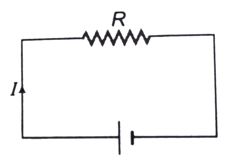
Assertion: If variation in resistance due to temperature is taken into consideration, then current in the circuit I and power produced across the resistance P both will decrease with time.
