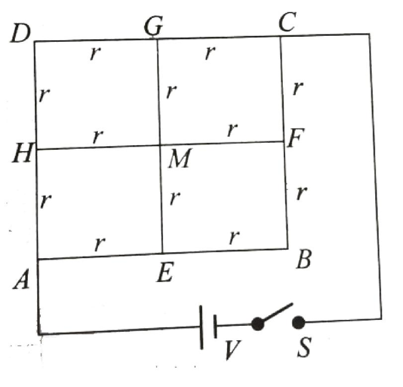
If a potentiometer circuit having gradient k is connected across the points H and C, the balancing length shown by the potentiometer is
