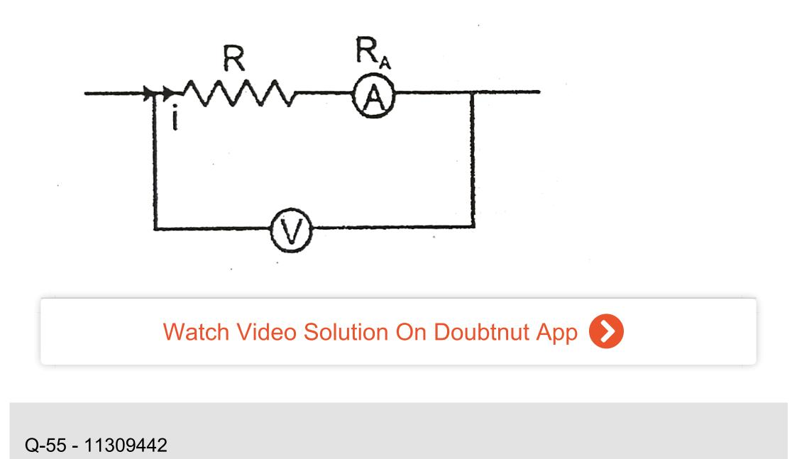
A battery of emf 1.4V and internal resistance  $2\Omega$  is connected to a resistor of  $100\omega$  resistance through an ammeter. This resistance of the ammeter is  $4/3\Omega$ . A voltmeter has also been connected to find the potential difference across the resistor.
