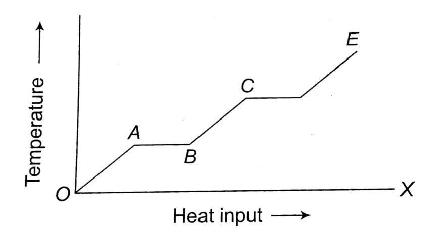
A solid material is supplied with heat at a constant rate. The temperature of the material is changing with heat input as shown (i) AB: change of state from solid to liquid.
