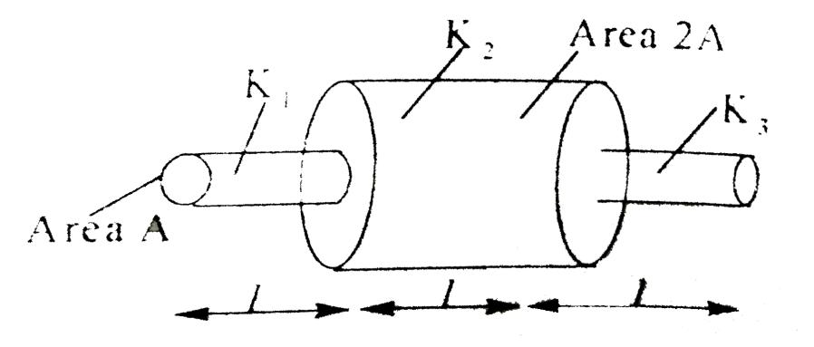
Equivalent thermal conductivity of figure given below will be given that length of eachh cylinder is l and area of cylinder having thermal conductivity  $K_1 \& K_3$  is A while middle cylinder is having  $K_2$ .
