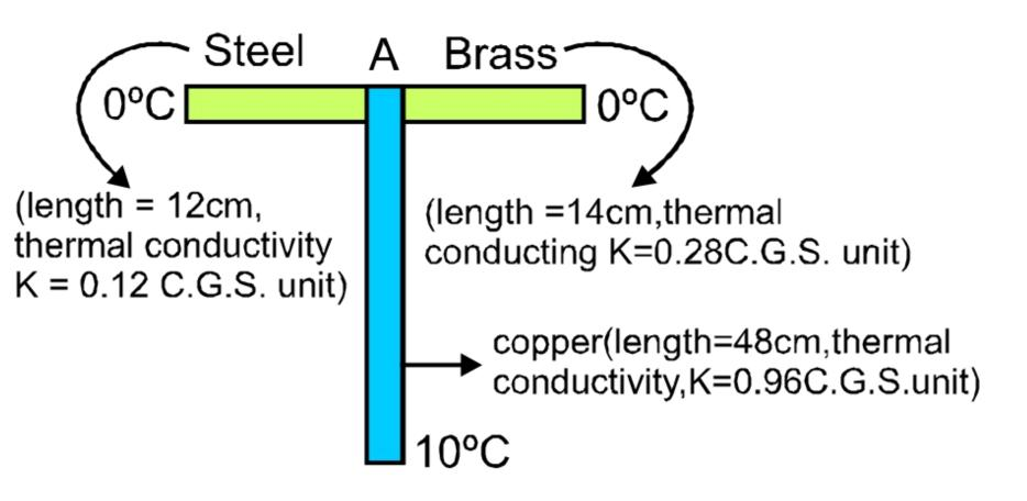
Three rods of copper, brass and steel are joined together to form T shape as shown in figure. The cross sectional area of each rod is  $4cm^2$  the end of copper rod is maintained at 10C and the ends of brass and steel rods at 0C assume there is no loss of heat to surrounding. What is temperature of junction point A in . C
